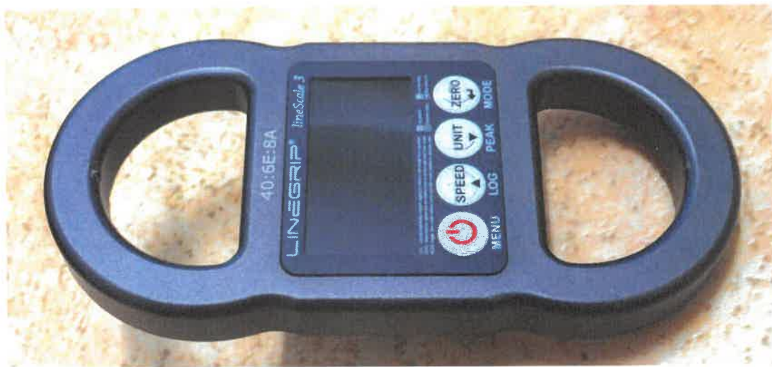
LineGrip LineScale-3, type Electronic Load Cell
