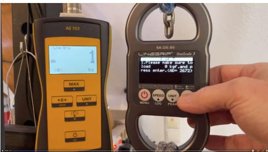
Ensure the LineScale is completely unloaded, then press enter.
