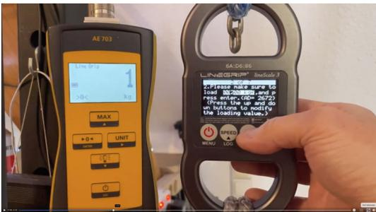
Confirm your change with the enter button. After the last digit the LineScale will exit the load edit mode, and wait for your confirmation to calibrate.
