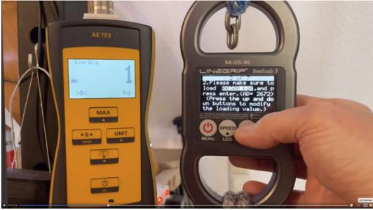
Then adjust the digit using the up/down buttons.
