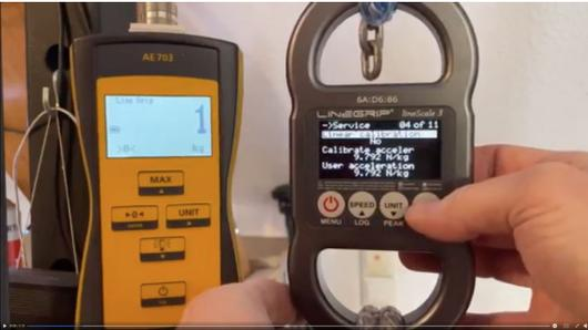
Scroll down to "Linear Calibration" and select with the enter button.
