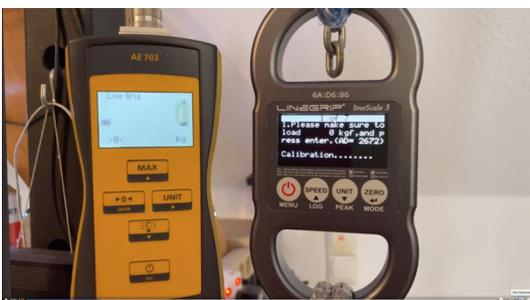
The LineScale is now calibrating the Zero-Point. Wait until the dotted line runs to the right.
