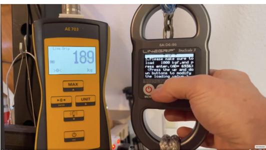
After this value is calibrated, the LineScale will ask for the next calibration value. In this case, value #2 is preset to 1000 kgf.
