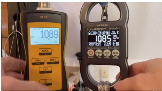
After the final calibration step, the LineScale will exit to the main screen, showing the current load in the preset unit. If you had the unit set to kN it will now display in kN again, so make sure to change your reference scale to this unit as well to verify the calibration.
