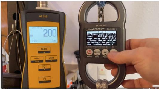
Increase the load to the set value and press the enter button to start calibrating this value.
