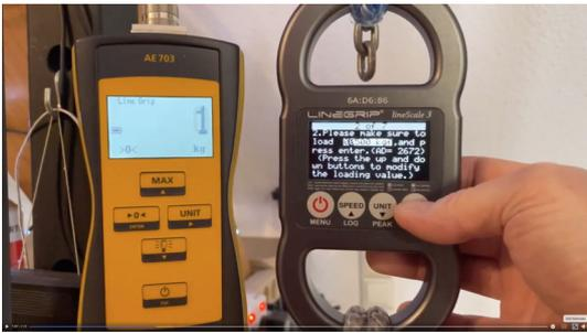
In load edit mode, scroll to the desired digit using the enter button.
