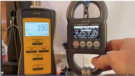
After the value is set, again confirm with enter, increase the load to the set value, and confirm the calibration start...
